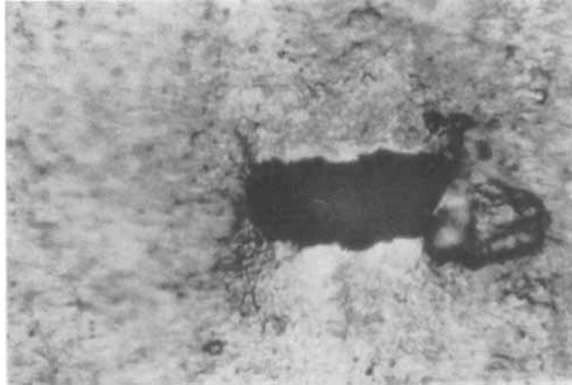
FIGURE 7 Shape of cracks. Ozonized BMSR rubber surface.
